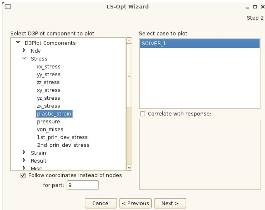
*Figure 20-17 For metal forming specify that the coordinates instead of the nodes must be followed and specify the part (blank) for which the results must be mapped.*
