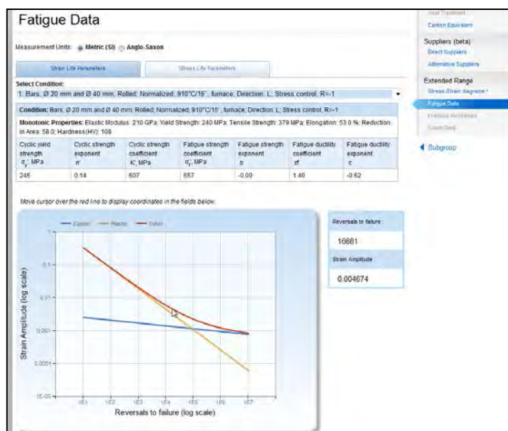
Fig. 3. An example of strain-life fatigue data. Monotonic properties are provided for reference.
